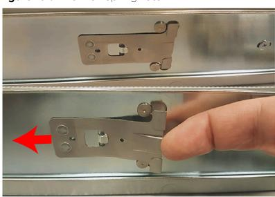
Figure 161: Inner Rail Spring Latch
