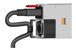
**Step 4:** Remove the power cable from the faulty PSU.
