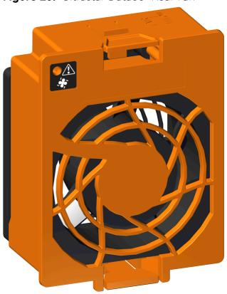
The Rear Fans are toolless modules that provide the primary system cooling for the Ultrastar Data60 . They are attached inside the fan housing at the rear of the chassis by two latches and a 6-pin connector, which also provides power and control signals to the modules.
