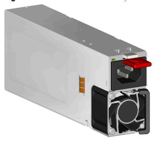
The Ultrastar Data60 contains redundant 1800W Power Supply Units (PSUs). Each Artesyn PSU requires an input voltage between 200 - 240 VAC. The Artesyn PSUs are 80 PLUS Platinum certified and utilize C14 power cable receptacles.
