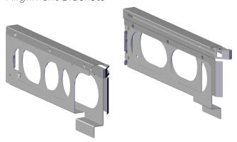
The Rear Cover Alignment Brackets are designed to keep the top cover of the Chassis in the rack while extending the Ultrastar Data60 out of the rack for servicing. The Rear Cover Alignment Brackets attach to the rear vertical rack rails and rest on top of the toolless rail system.
