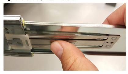
**e.** As the chassis is slid into the rack, position one installer at the rear of the rack to ensure that the pegs on the sides of the cover will slide correctly into the rear cover alignment brackets on both sides of the rack. If the chassis does not install smoothly or snags, check that the rear cover alignment brackets are not interfering with the chassis sidewalls, and try again.
