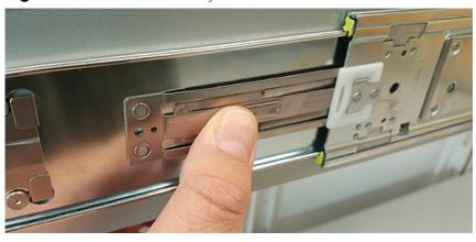
**Step 10:** Remove the chassis from the rack.
