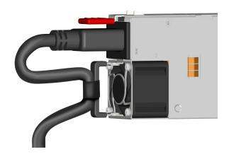
**Step 8:** Make sure the CMA(s) is in operational position by folding the arm(s) in toward the enclosure and attaching the elbow end(s) to the connector(s) attached to the rail. Verify that all of the cabling is in functional order and does not bind or catch.
