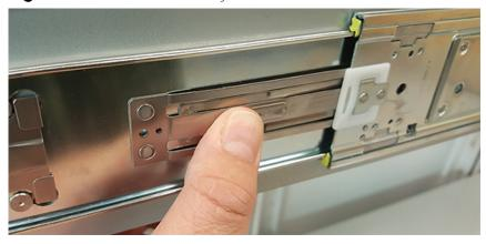
**Step 19:** Push the chassis back into the rack.
